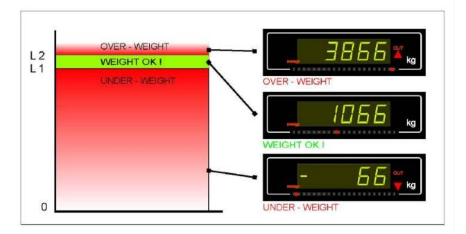
The Indicator shows: Underweight by the arrow point down and a dot on the left side of the led-bar. Overweight by the arrow point up and a dot on the right side of the led-bar. When the weight is correct we find the dot somewhere in the middle of the led-bar. The led-bar dimension is scaled to the weight OK-band. These indications are there for maximum 1 second or are instantly refreshed by a new value.
